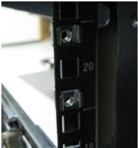
Attach the rear ear to the cage nuts using the long screws. Please note the orientation of the ear in the photo. The protruding mounting hole should be placed toward the top.
